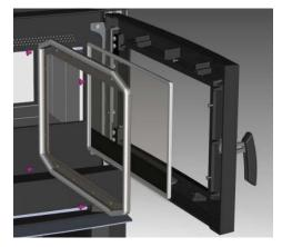
7) Flip the handle around 180° and reattach to the door with 2 botls.
