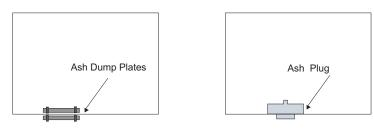
4) Push the ash plug into the hole inside the firebox and replace all the bricks except for the brick over the ash plug. See brick diagrams in manual.
