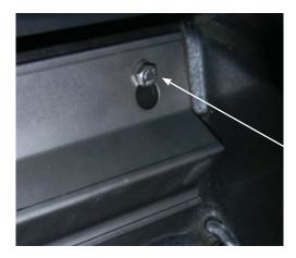
Ensure defector is seated so bolts are situated at the top of the keyhole before tightening.
