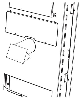
4) Slide cap over end to pipe to complete the installation.
