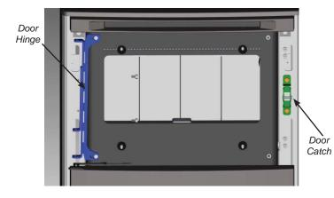
6) Remove the glass from the door and flip it around 180° - so the painted strip is at the bottom of the door.
