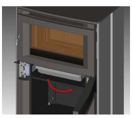
2) Ashlip to be positioned just below the ashdrawer (if installed).
