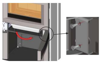
2) Remove and discard the latch on the left side of the unit by removing 2 bolts.
