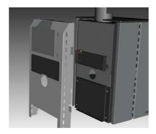
2) Center the plate / pipe over the opening on the back of the stove. Secure with 4 self tapping screws.
