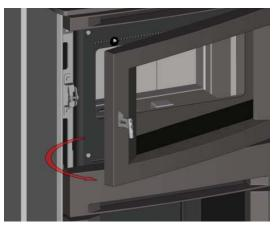
2) Remove the 2 bolts securing the door hinge to the unit.
