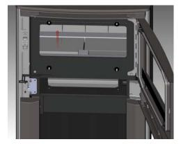
2) Remove the bricks from the floor of the firebox.
