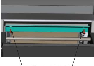
Smoke deflector installed with 2 bolts.
