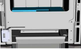
3) Remove the ash dump cover plates (one inside the firebox and one on the underside of the firebox - access the lower plate through the center door - it is directly below the upper ash dump plate.) by removing the two nuts and bolts holding the 2 plates together from underneath the stove.
